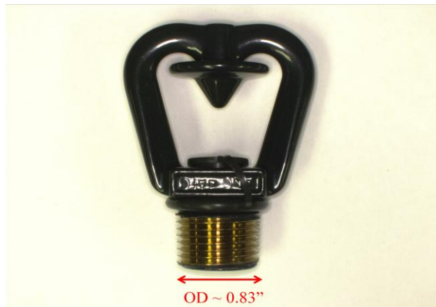
Figure 6.6 Photograph showing a corrosion-resistant nozzle with ethylene chlorotrifluoroethylene (ECTFE) coating, rounded deflector, and Teflon-based plug.
