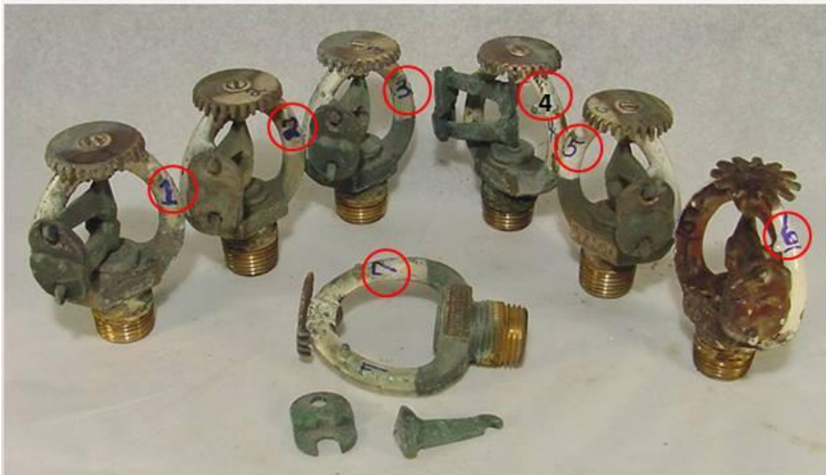
Figure 5.13 Photograph showing six intact (top, #1-6) and one prematurely operated (bottom, #7) sprinkler heads. The #7 sprinkler's fusible link halves had separated during the premature operation incident.
