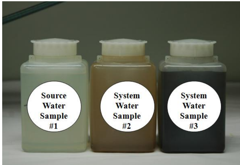
Figure 5.11 Photograph showing the three water samples in a wet pipe system. Sample #1 is from source water. Samples #2 and #3 are system water samples.
