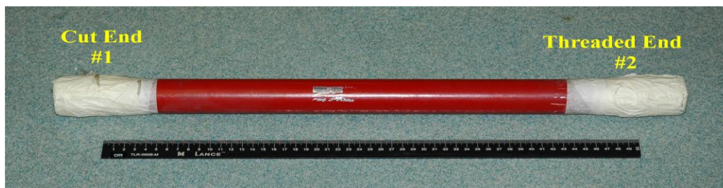
Figure 5.12 Photograph showing an NPS 1¼ branch line pipe sample.
