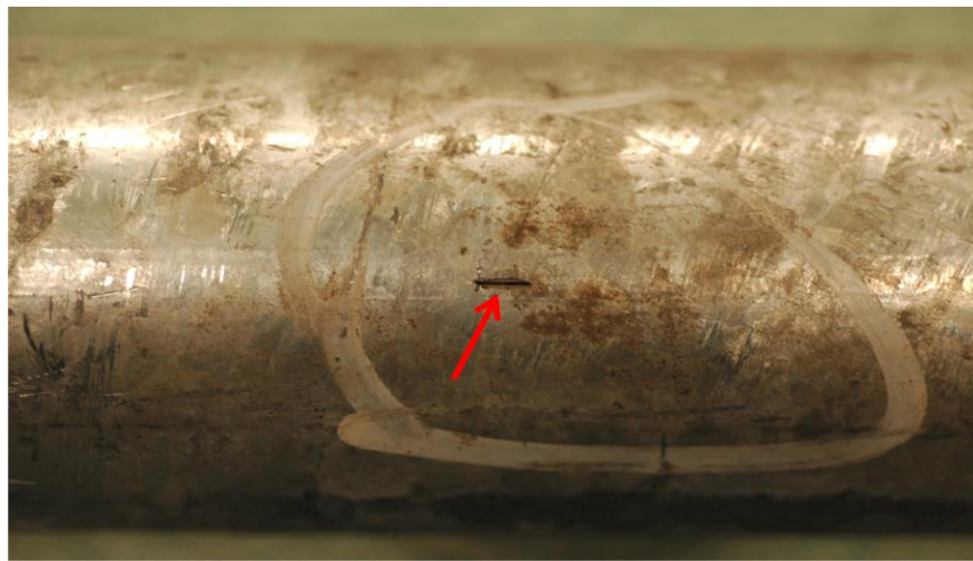
Figure 5.4 Photograph showing preferential grooving attack surrounding the weld seam area in a preaction system.
