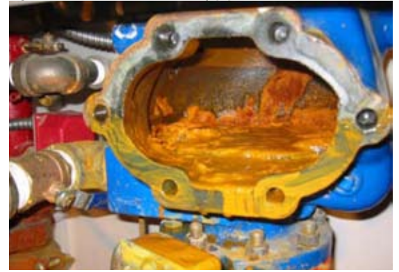
Figure 6 Corrosion inside a galvanized steel sprinkler pipe
