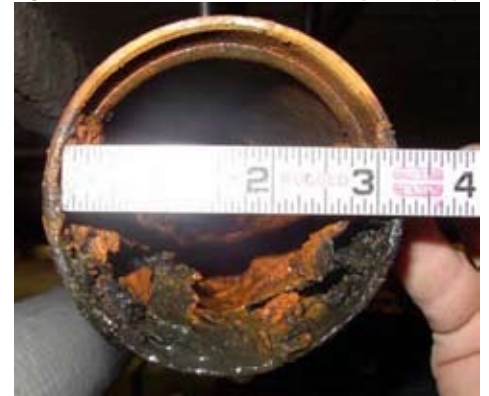
Figure 7 Corrosion inside a black steel sprinkler pipe
