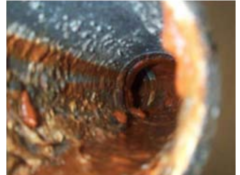
Figure 7 Corrosion inside a black steel sprinkler pipe
