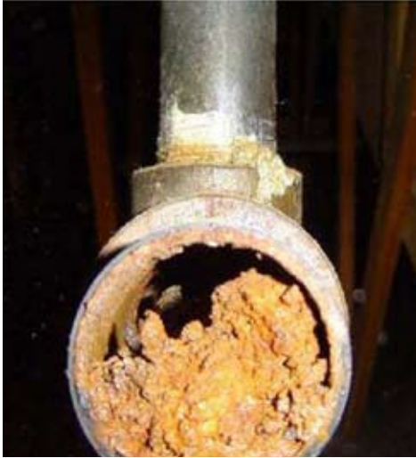
Figure 9 Corrosion products removed from a dry pipe sprinkler system
