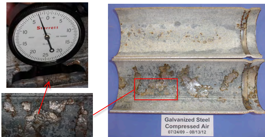
Figure 5. Galvanized piping after 1116 days exposure while approximately half-filled with water and under compressed air supervision. Note localized pitting at locations where zinc coating has been breached.
